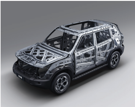
SAFE BODY STRUCTURE 85% HIGH-STRENGTH STEEL
